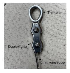
Duplex grips are not suitable for use with construction cables or lifting applications.
